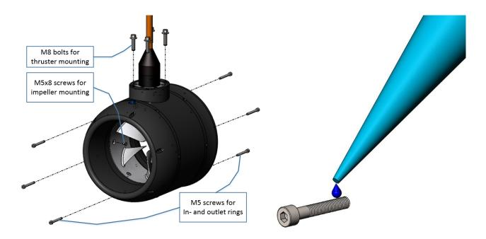
If a thruster bolt or a screw has to be changed, swapped or re-fixed, always add a bit of AquaShield grease on the thread. Use a torque wrench to make sure the screws are properly tighten according to the following values:
