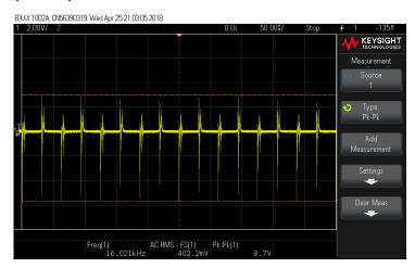
Most analog converters have a low pass filter good enough to make the signal from the Pt1000 sensor stable and usable to read temperature. If this is not the case and the noise is too high, it is then recommended to consider the use of a small capacitor in parallel with the analog converter input. See Figure below.
