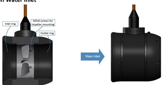
To detect the main water inlet side of the thruster, look for the screws on the inside of the propeller. The main water inlet is on the opposite side of the propeller blades from these screws.
