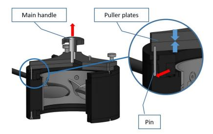
• Make sure that the main handle is fully retracted, that the puller plates are close together, and that the 3 pins stand firmly on the bottom of the screw holes.
