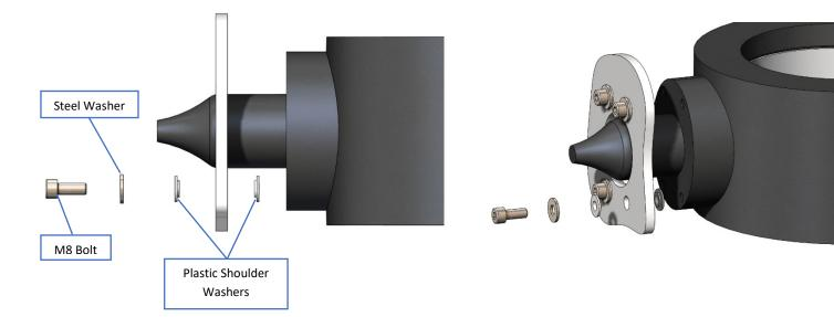
• If the mounting bracket is too thin to insert a shoulder washer in both sides on the mounting bracket – the following set of washers are needed: (1x plastic shoulder washer & 1x flat plastic washer)
